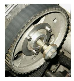
For advancing, or clockwise adjustment, slide needle into the hole that corresponds to the amount of advance desired.
