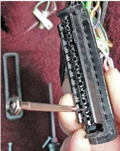
Push in to release terminal catch (#12) as shown.
