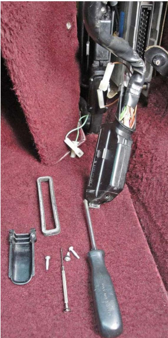
Disconnect plug from LH. (*Tip: push in at wire harness end when releasing spring catch*)
