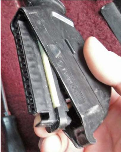
Lever the terminal assembly out of its case.
